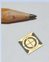
Figure 1. The BLU energy transducer is a small form factor device that can generate ultrasonic forces powerful enough to shear DNA without cavitation. It is readily scalable to meet high-throughput sample preparation needs by utilizing parallel, simultaneous channels.
